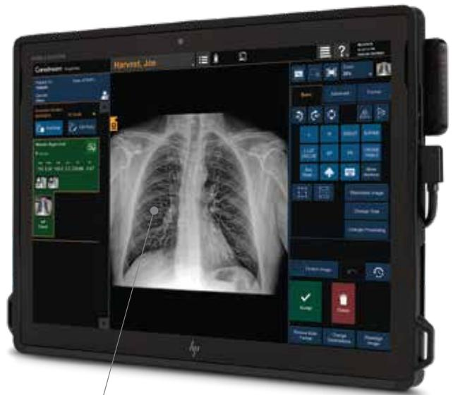
The DRX-Transportable System/Lite features wireless tablet operation. There's no bulky electronics box required, and no need to work from a fixed console – you can move freely around the exam room. A DR Detector and battery charger complete the system.
